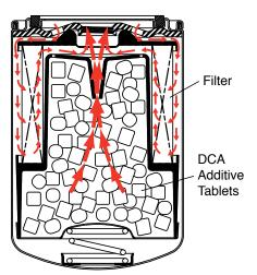
Fleetguard® ESI water filters are specifically designed to release the proper amount of coolant additive in order to provide the appropriate coolant system protection over time through a patented coated tablet technology. These tablets are held in a special chamber which prevents the tablets from dissolving too quickly and introducing excess additive into the coolant system.
